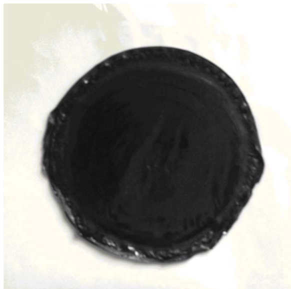
Figure 3. Picture of the PVA/KE-4BD PEM prepared by solution-casting technology with a plastic Petri dish as a container. [Color figure can be viewed in the online issue, which is available at wileyonlinelibrary.com .]
